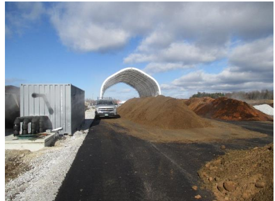
Compost windrows on the new VT Natural Ag Products working pad in November 2017 with Agrilab Technologies Hot Box 250-R CAHR unit at left.
